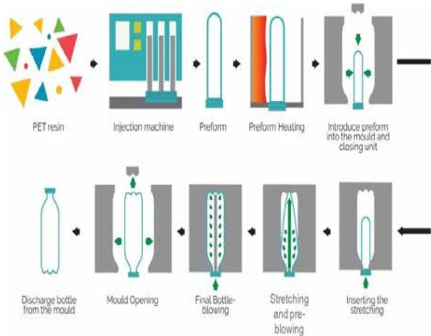
Figure 3: Preform Manufacturing Process
